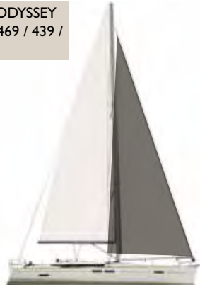
Short overlapping genoa Performance / Génôis Performance à faible recouvrement / Genua in geringer Überlappung Performance / Génova con poco recubrimiento Performance / Genoa a basso recupero Performance
